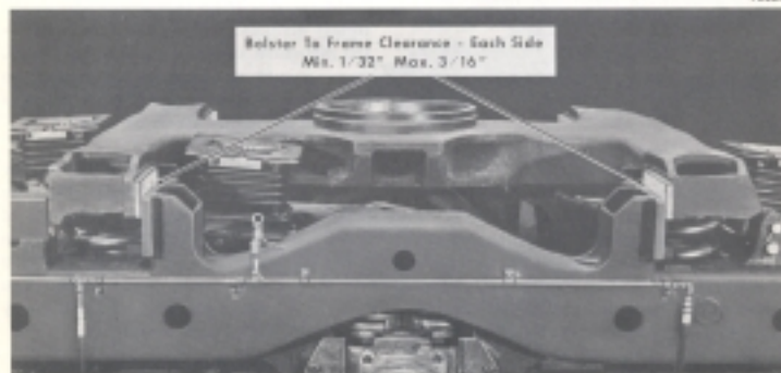
Fig. 10 - Current SD Bolster Wear Plates
