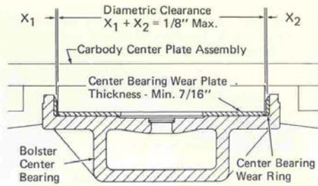
Fig. 7 - Center Bearing Wear Plate And Wear Ring Limits
